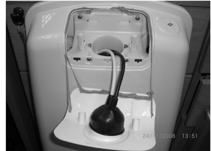
Locate the 4 screws holding the panel in place and remove with a cross head screwdriver as seen in illustration E
