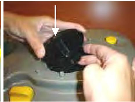
Press the new blade gently in the hole of the blade arm.
