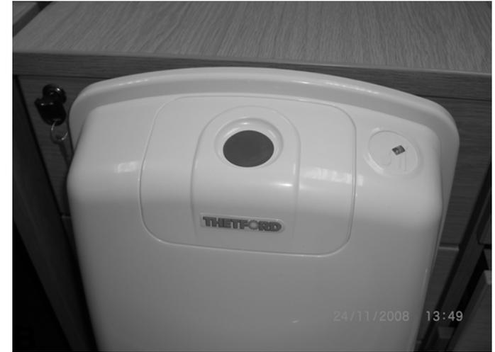
Use a paint scraper type object (use a cloth around the scraper if necessary to prevent damage to the toilet) and lever up the bezel, slowly working the bezel free all the way round. Illustration C
