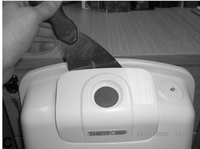
Once removed you will be able to turn the bezel over revealing the retainer panel.
