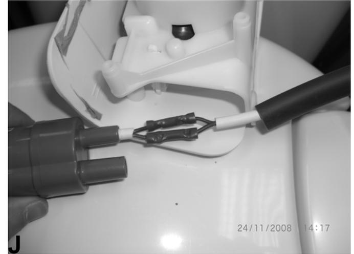
Slide the heat shrink back over the newly made connection and apply the heat evenly over the shrink ensuring the connection is covered and water tight. Illustration K
