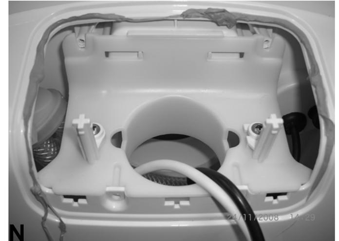
Replace the bezel. If required use some of the PTI sealant provided ensuring a nice clean seal.
