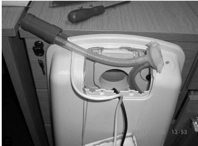
Disconnect the flush tube from the pump. Cut the wire approximately 50mm from the pump. As seen in picture H
