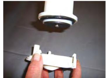
Place new pump retainer and press it back onto the pump.
