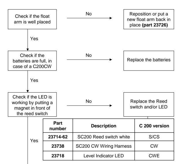
Reposition the reed switch closer to the holding tank
