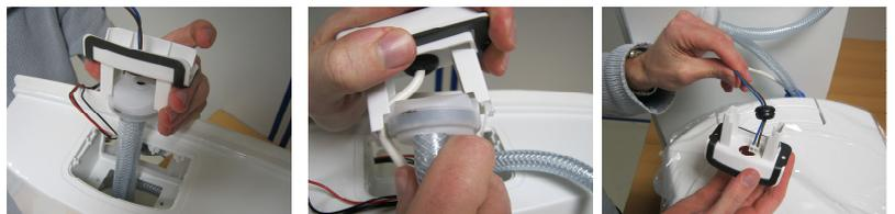
Pull water tube of the pump.
