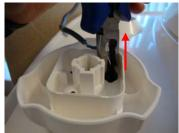
Fit plug onto new control knob.
